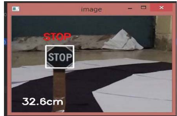
Figure-6.10 Detected stop sign with distance measurement
